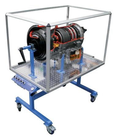
The ConsuLab EC-1106-3 cutaway Allison transmission has been specifically designed for teaching heavy duty automatic transmission theory and operation. It has been strategically sectioned and cutaway to allow students to visualize the internal transmission functions. The Allison 3000 series is a fully automatic torque converter driven, electronically controlled 6-speed automatic transmission that is commonly used in coaches and heavy vehicles. The other Allison Series are available on request.
