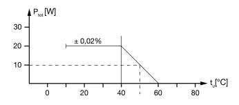
The max. load capacity with different ambient temperature as a function of the warm-up error can be taken from the load reduction curve. <u>Example:</u> Ambient temperature: max.  $50^{\circ}$ C; accepted  $\triangle$  R by temperature influence: max.  $0.02^{\circ}$ ; max. permissible load:  $10^{\circ}$ W.
