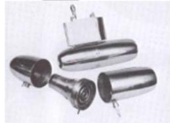
The ramjet engine is fabricated from a heat resistant alloy and requires no maintenance even after many years of operation.
